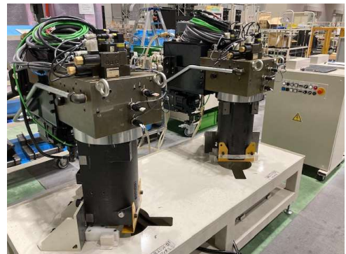
Automation of HRB D-axis module (hydraulic system) degassing
