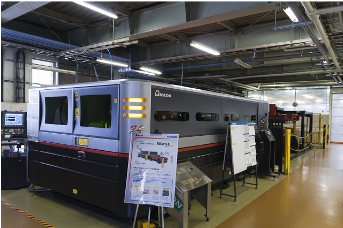
The FOL-3015AJ fiber laser machine (with shuttle table fitted) at the Orion Machinery Co., Ltd plant
