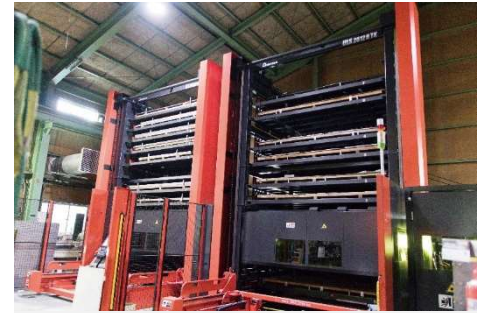
To work on work style reforms, they installed the EML-2512AJ with full-options, equipped with a PDC (automatic tool changer ), eight shelves for materials and a TK (takeout loader).
