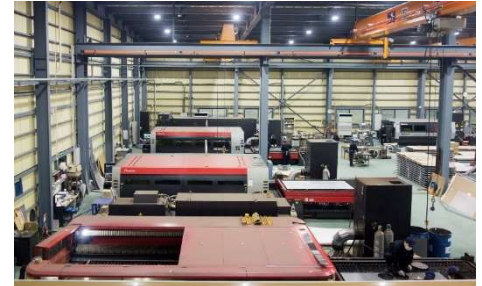
Three fiber laser machines and two CO 2 laser machines in line
