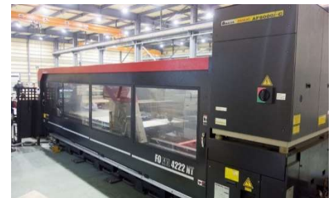
The CO 2 laser machine, the FO-M II 4222 NT (6kW), is mostly used for thick plate fabrication
