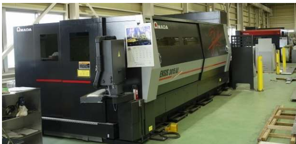
Inside the laser factory. Front: ENSIS-3015AJ (3kW) Rear: FO-M II R13015
