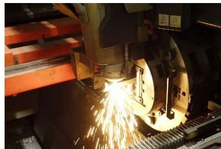
Square pipe laser processing using FO-M II R13015
