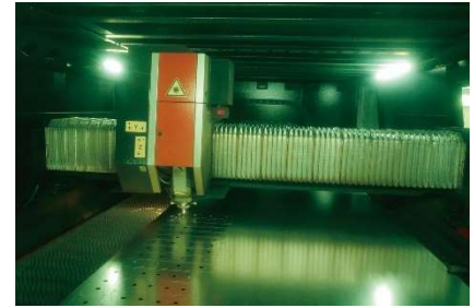
Processing hot-dip zinc alloy coated steel sheets with the ENSIS-3015AJ
