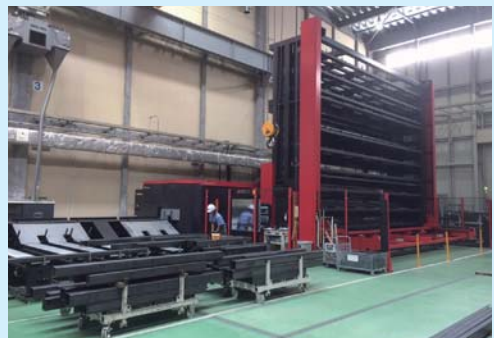
Pipe processing automation system
