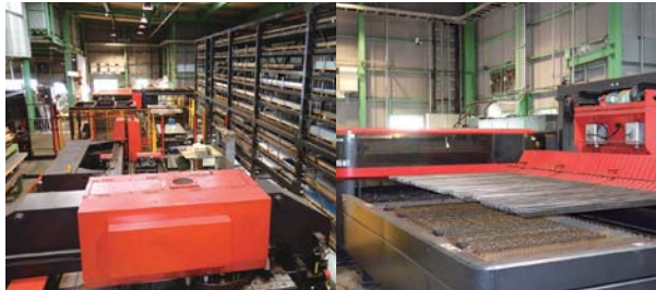
Left: A total of 3 machines, 2 laser machines and 1 punching machine, are linked in the Automated Warehouse MARS Right: Laser machines FOL-3015NT + LSC-3015FOL + LST-3015FOL
