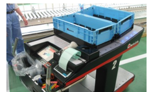
Bucket with IC chip inside, and picking cart with monitor (Parts Center)
