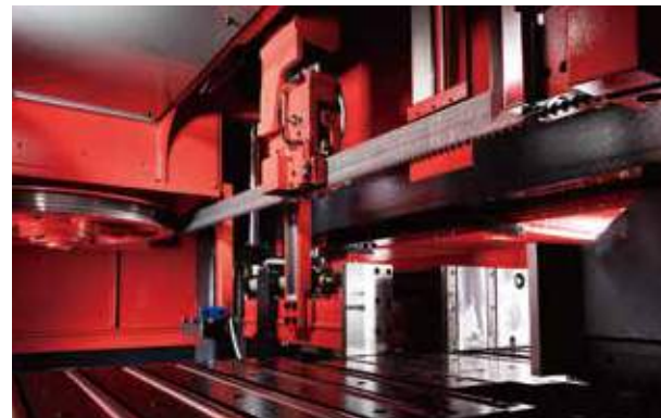
New saw head precision with a twist angle of zero degrees
