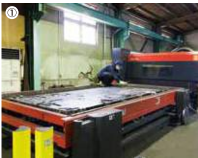
① CO 2 laser machine FO-MII4222NT(4 kW) capable of supporting 4x2m plate with thickness of up to 22 mm. / ② Nesting data for FO-MII. Nesting multiple parts in parts with no gaps on SPH 5' x 10' plate with thickness of 6mm.
