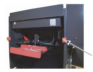
The EMERGENCY STOP buttons for working at the rear of the machine.
