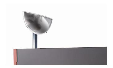
The rear-view mirror is used by the shearing machine operator to check the situation at the rear of the machine and the access of other operators to the rear of the machine.
