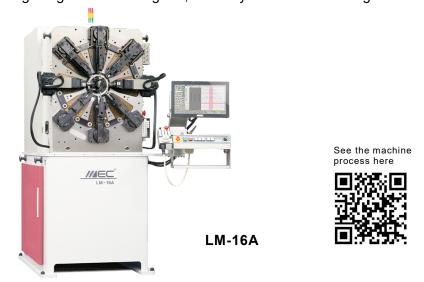
**AMADA PRESS SYSTEM CO., LTD.** (*Isehara, Kanagawa, Japan*) will launch sales of the "**LM-16A**" beginning March 8th. The LM-16A is a wire rotation torsion spring machine with a wire-rotating mechanism, eight processing slides, and 15-axis control. Torsion spring machines are spring formers that specialize in torsion springs, but can also be used for all types of wire processing forming including extension, compression and other spring forms.
