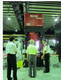
Observing how the power consumption of the press machine is reduced through the use of a servo motor and the fact that lubrication oil can be used continuously for one year
