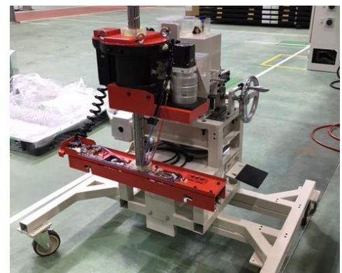
HRB ATC module punch lifter assembly table
