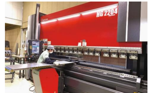
HG-2204 is one of the machines that are supporting their bending work.
