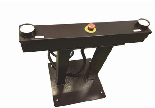
A stand-type control device with two-hand control push buttons.
