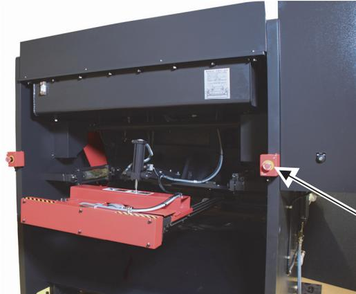
The EMERGENCY STOP buttons for working at the rear of the machine.
